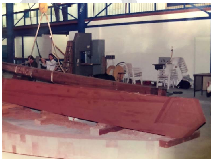
Figure 25. Keel of Endeavour replica showing the exposed keel-stem scarph (HM Bark Endeavour Foundation, Australian National Maritime Museum Collection).
