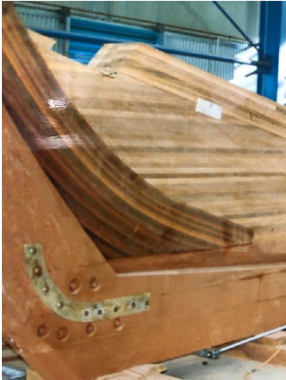
Figure 26. Endeavour replica stem and keel after being joined, showing the scarph, bolt pattern, and modified horseshoe plate (HM Bark Endeavour Foundation, Australian National Maritime Museum Collection).
